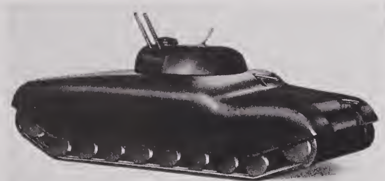
FIGURE 2. Model of IVI-C medium tank equipped with two 37-mm guns.
